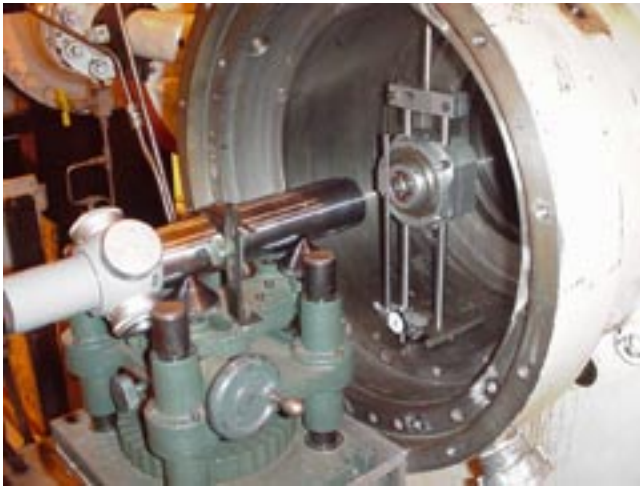
Picture Two, Adjustable target holders installed in crosshead guide
